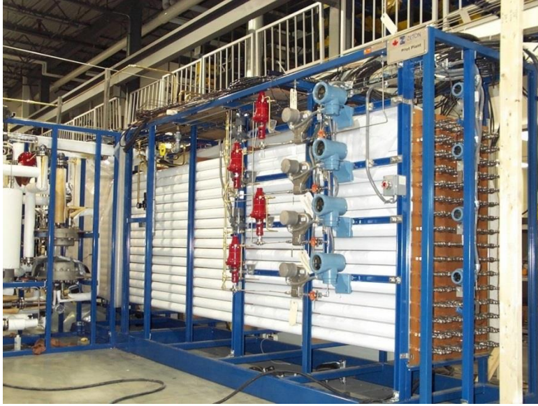
An example of a pilot-scale PFR for a confidential client and process
