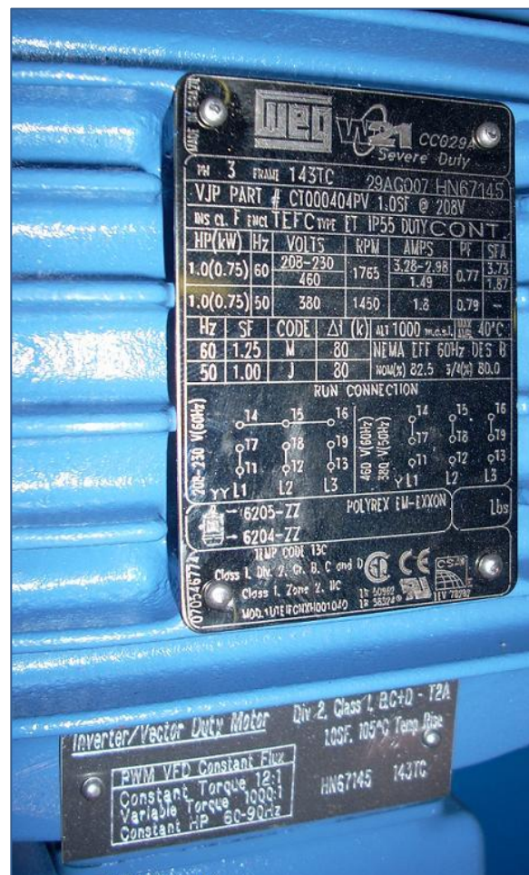
Figure 1. Inverter-duty motor nameplate for Class I, Division 2, Group B, C, and D.
