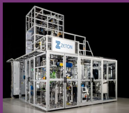
A plastics de-inking plant
