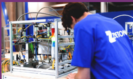
Factory testing of a ContiUnity® module in Zeton's shop
