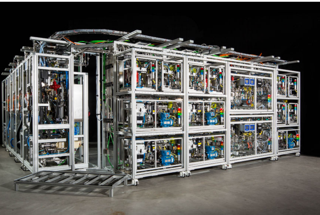
A modular pilot plant for the continuous production of APIs
