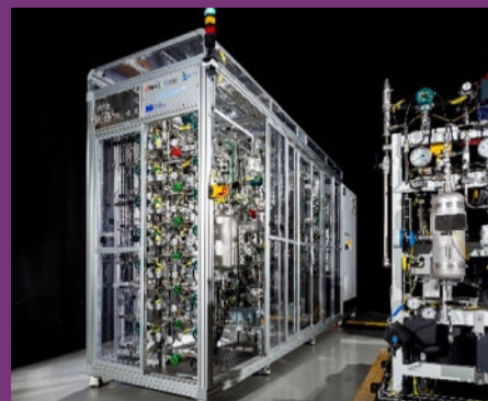
A CO 2 to fuels and olefins conversion pilot plant
