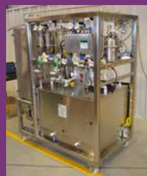
A reagent dosing skid in a pharmaceutical industry application
