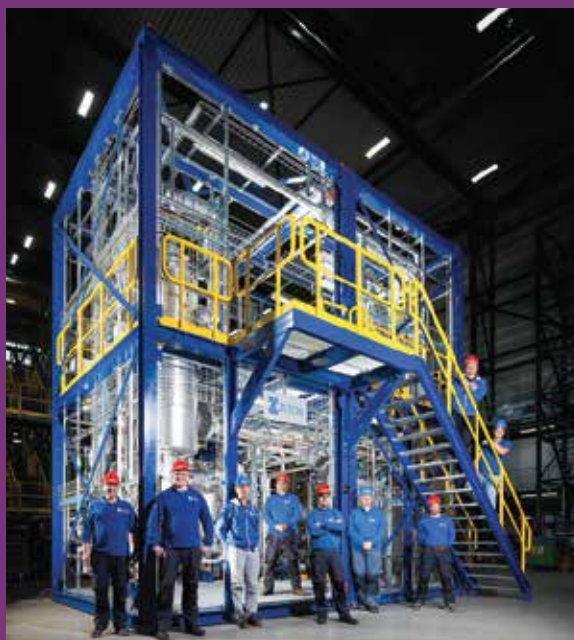
A separation skid in a biofuels industry application
