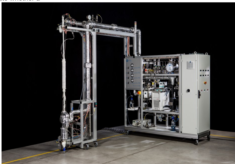
Figure 1. A lab scale gas-to-liquids catalyst test system
