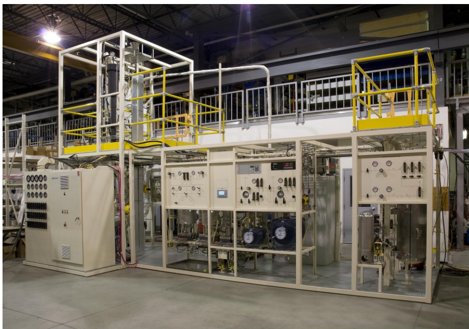
Figure 4. A Grace DCR fluidized catalytic cracking (FCC) pilot plant
