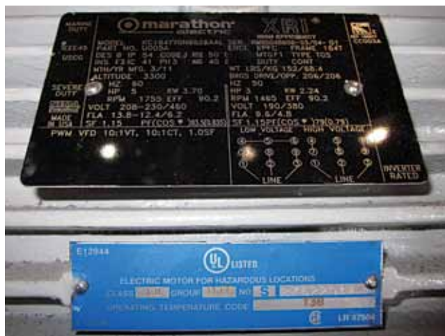
▲ Figure 2. This nameplate indicates that the motor in Figure 1 is rated for use in a Class I, Group D location and has a T-code rating of T3B. Note that the motor is also rated for use in a Class II environment.
