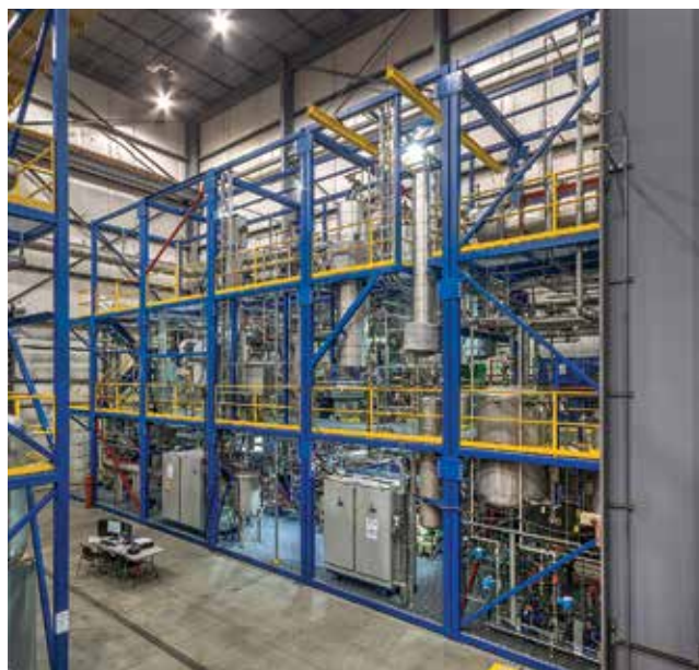
▲ Figure 5. This oil production facility consists of multiple operating trains. The producer was able to increase capacity by adding additional units instead of initially building one large unit.
