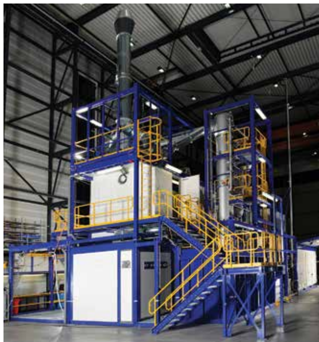
▲ Figure 3. To reduce the risk of transporting hazardous chemical products, modular plants can be located at their point of use. This modular plant produces a hazardous chemical that is used at the site, and it can be relocated with ease and at minimal cost.
