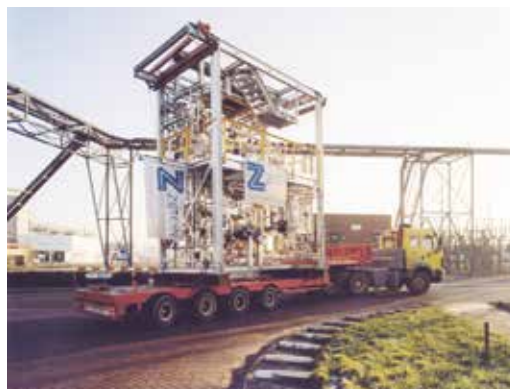
▲ Figure 2. Careful consideration is required when deciding whether to take the modular approach. For example, road transportation may be subject to width, height, and/or weight limits, which may direct the route available for transporting modules to the manufacturing site or prevent the use of trucks.
