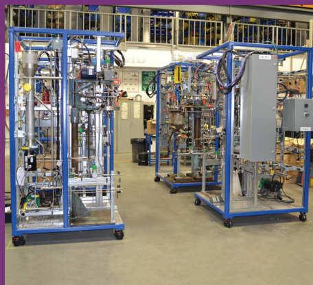
A laboratory mix tank system
