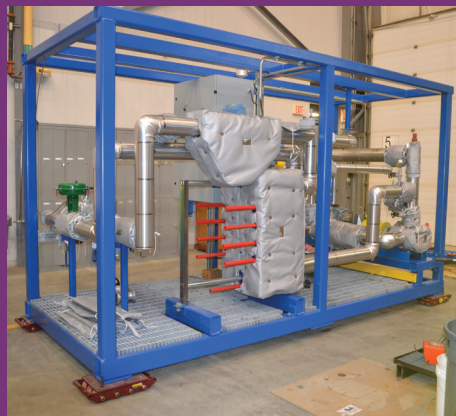
A Canola oil injection skid
