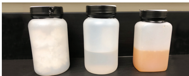
Wax, Diesel, and Water product from the first operation of the CTL Facility
