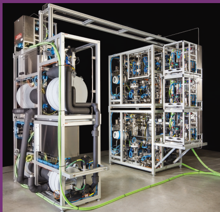
A continuous pharma modular Plug-and-Produce manufacturing plant
