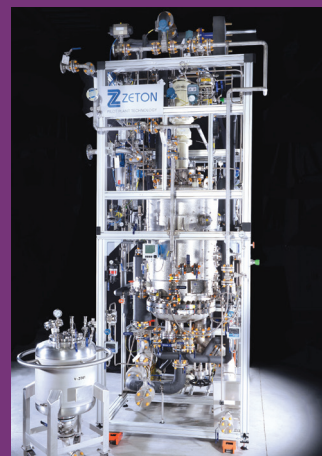
A polymer coagulation pilot plant
