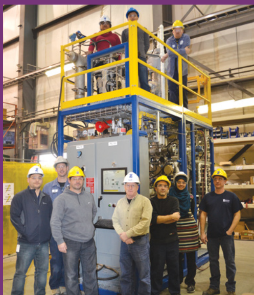
A free fatty acid pyrolysis pilot plant
