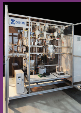
A bio-oil microactivity test (MAT) unit
