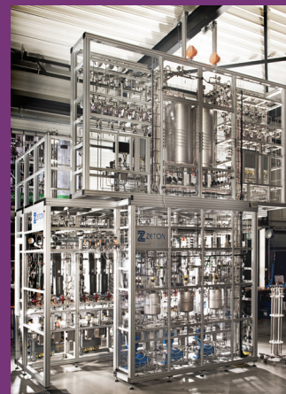
A multi-reactor catalyst test unit
