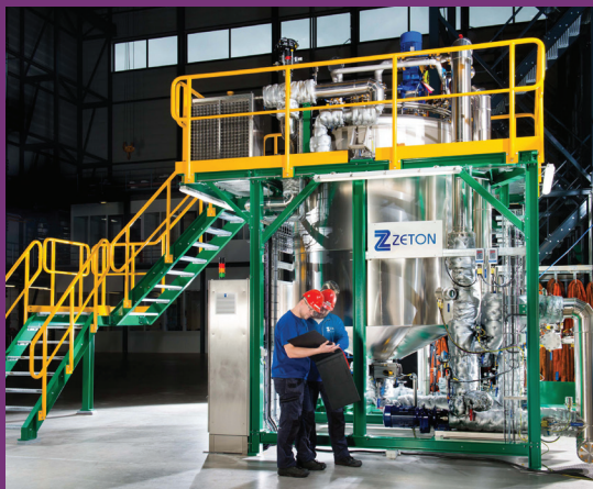
An oil blending pilot plant
