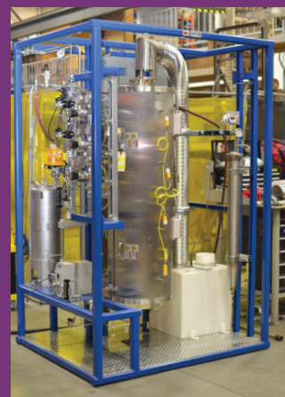
A 10 kg FCC catalyst steam deactivation unit with CPS
