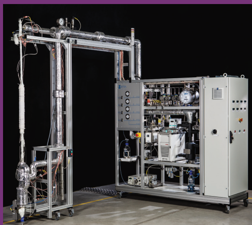
A lab scale GTL catalyst test system
