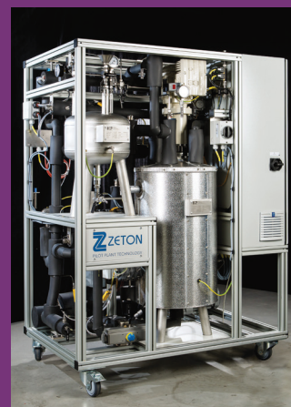
An oil filtration module
