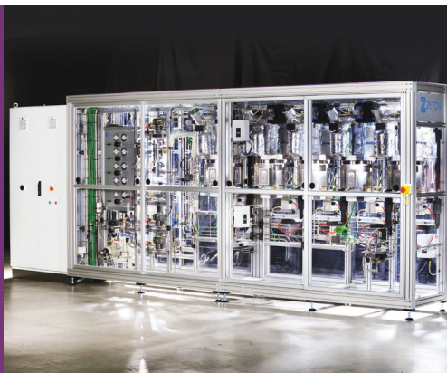
A bench scale chemicals catalyst testing unit
