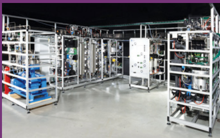
A hydrotreater pilot plant for a customer in Russia
