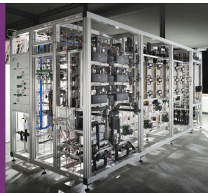
A high throughput testing plant with 12 parallel reactors
