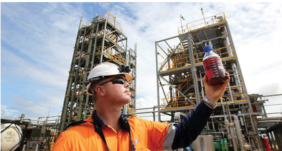
QER's Jason Pringle with a sample of the intermediate raw distillate product from the Oil Upgrader Plant. This material is the feedstock for operation of the higher-pressure Mode 2 operation that produces retail quality ULSD (Photo courtesy of Queensland Energy Resources).
