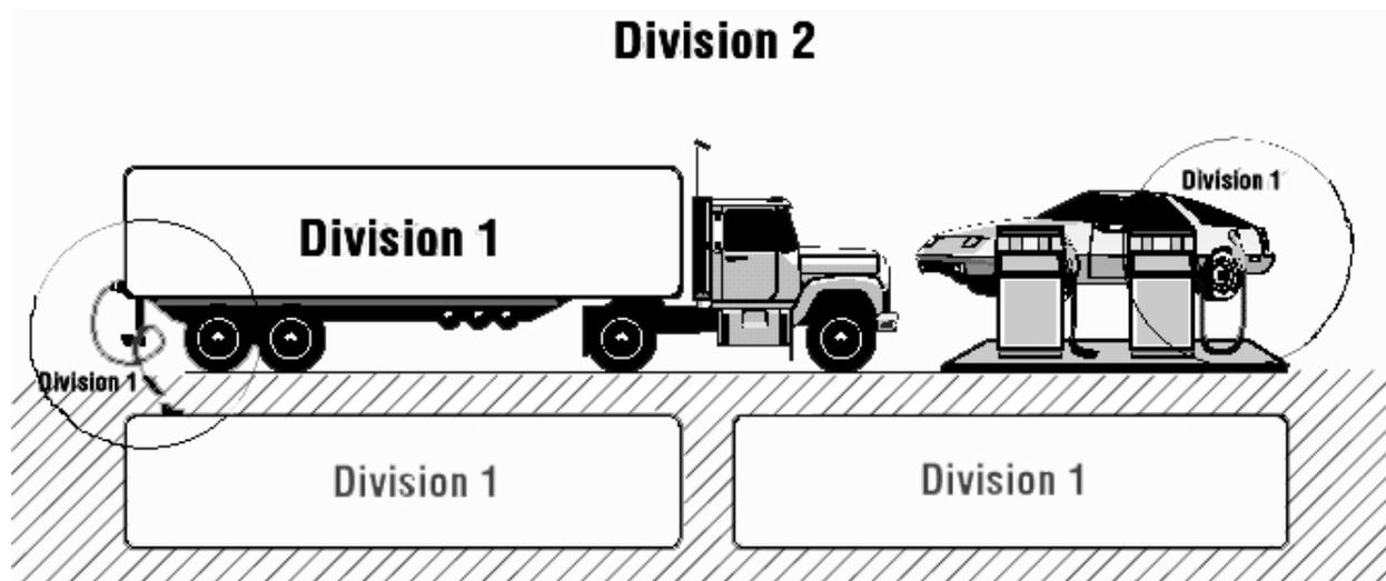
Figure 1. FOR ILLUSTRATION PURPOSES ONLY. The Division 1 areas are those that contain ignitable materials under normal operating conditions. The Division 2 area is defined as containing ignitable materials only under abnormal conditions (e.g., a leak).
