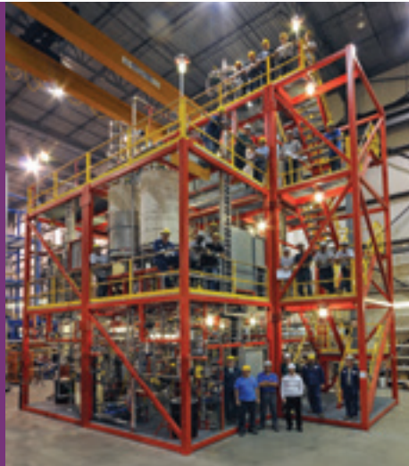
A Rapid Thermal Processing (RTP™) Integrated Biorefinery (IBR) demonstration plant
