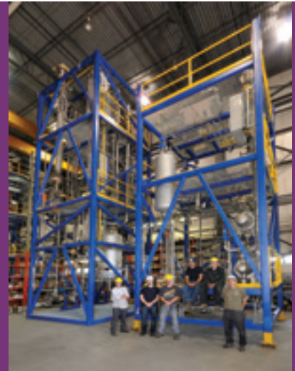
A syngas to green gasoline Integrated Biorefinery (IBR) demonstration plant
