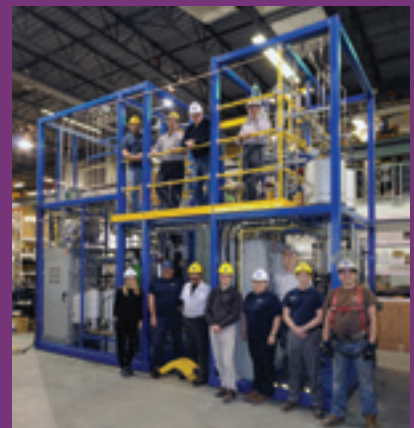
Bio-oil upgrader pilot plant with product fractionation
