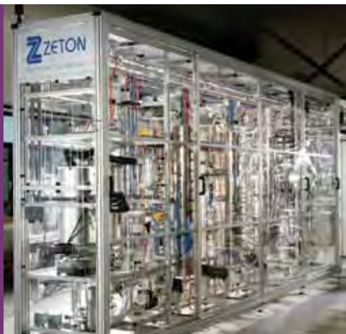
A four reactor hydroprocessing pilot plant
