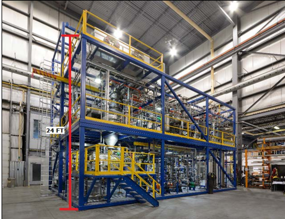
Figure 4. Two-story pilot plant, with entire plant fitting into pool fire.
