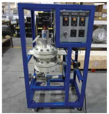
A custom-designed lab scale solids feeder capable of feeding biomass (wood) at a nominal feedrate of 100g/hr at pressures up to 700 psi
