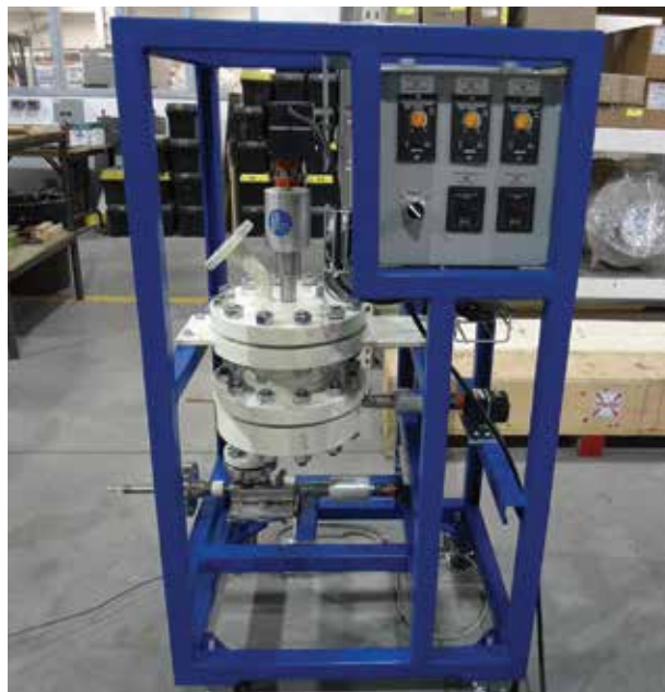
▲ Figure 3. Solids handling should be carefully considered as early as possible in the development of biofuels technologies. A lab-scale (100-g/hr) pressurized feed system is shown here. Photo courtesy of Zeton.
