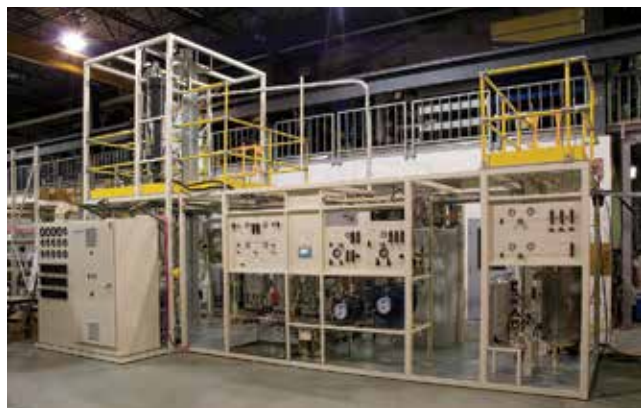
▲ Figure 4. A traditional CPI pilot plant has been modified to include a continuous biomass feed system. Photo courtesy of Zeton.
