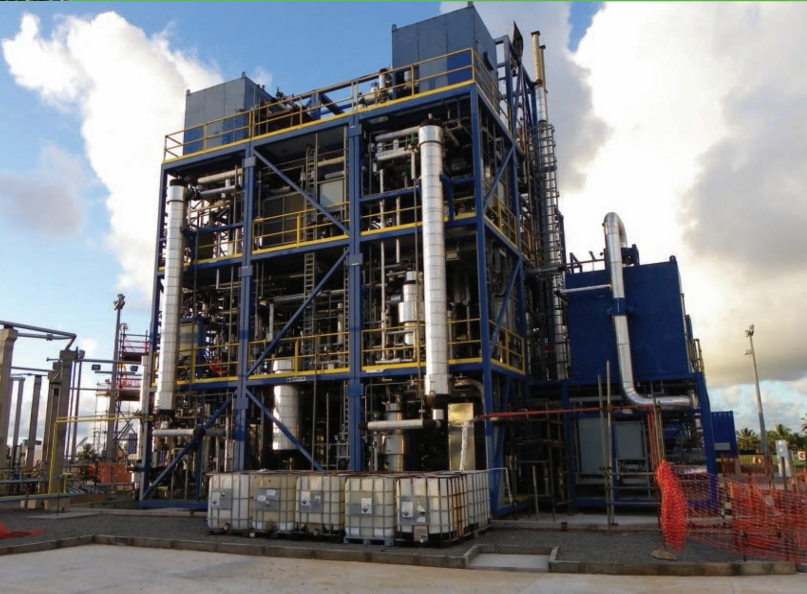
Zeton designed and built the world's first modular gas-to-liquids (GTL) commercial demonstration plant using Compact GTL's mini-channel reactor technology. The USD 20 million plant incorporated all aspects required for commercial application in treating gas at remote and offshore oil fields. Access to a real-time 3D model during fabrication improved accuracy and reduced rework.
