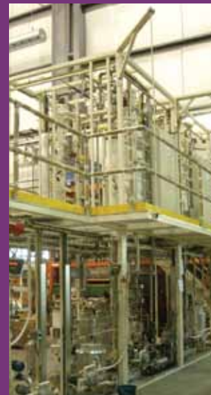
Continuous distillation pilot plant for Ecopetrol in Colombia
